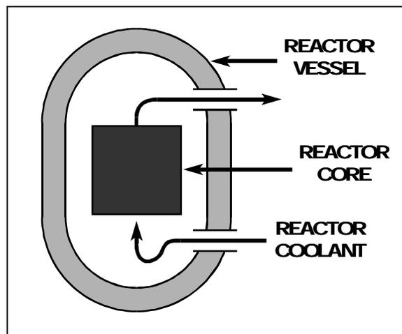
**Core, Vessel, and Coolant**
