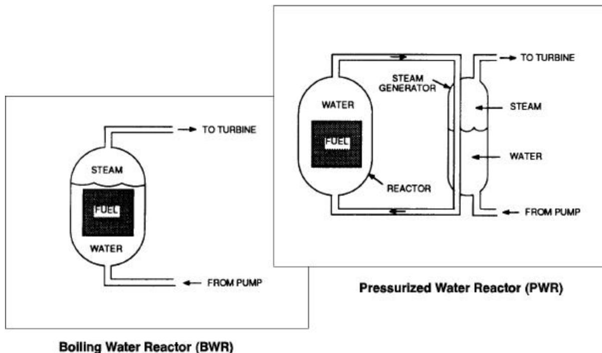
In Boiling Water Reactors (BWRs), water (primary coolant) is allowed to boil directly in the reactor core. The boiling water generates steam which is drawn away from the reactor and used to rotate the turbine, which in turn generates electricity via the generator. Even in non-emergency conditions this water may contain small amounts of radioactive fission products.
